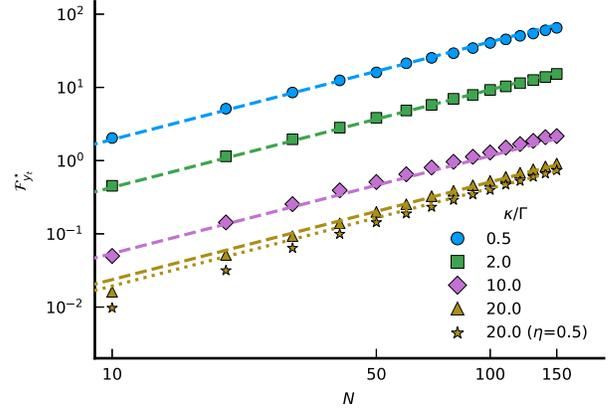
FIG. 4. Continuous monitoring FI  $\max_t[\mathcal{F}_{y_i}/t]$  (markers) as a function of  $N$  for different values of the dephasing rate, with  $\omega/\Gamma = 10^{-2}$  and number of trajectories  $n_{\text{traj}} = 10000$ . Dashed lines showing superlinear functions scaling as  $N^{4/3}$  have been plotted as a guide to the eye.
